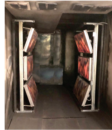
Retrofitted IR rack system
